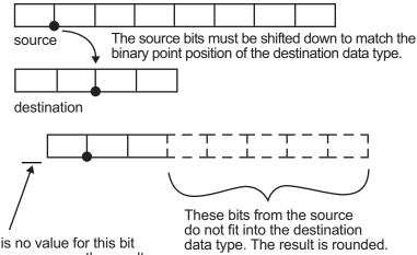
There is no value for this bit from the source, so the result must be sign-extended to fill the destination data type.
