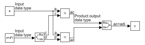
**Complex-Complex Multiplication.** The following diagram shows the multiplication of two complex fixed-point numbers in Fixed-Point Toolbox. Note that the output of the multiplication is in the sum data type, which is governed by the fimath SumMode property. The product data type is determined by the fimath ProductMode property:
